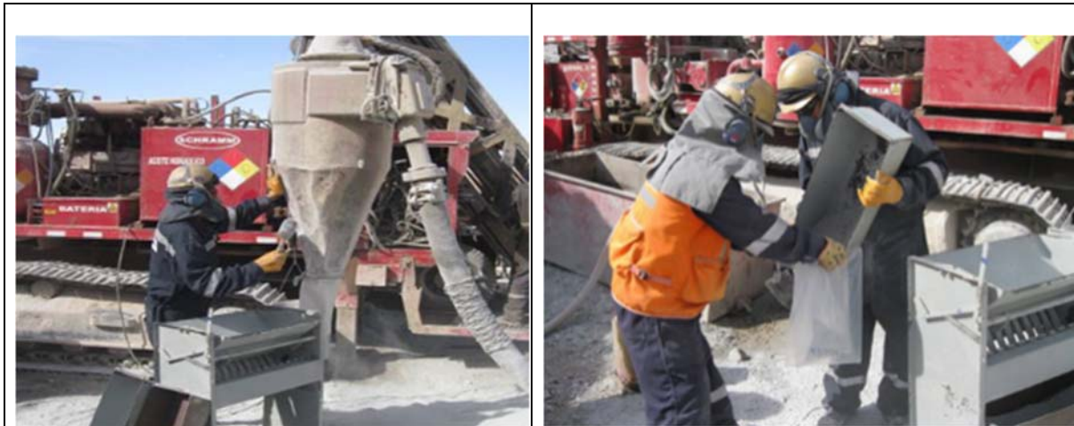
Figure 20: Photographs of the sampling at the RC drill rig
